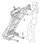
• To transport, hold the treadmill from F position and tilt until the wheels are able to move on the ground.
