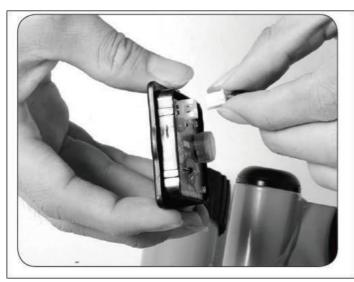
Connect the Computer (Part: 22) with Main Frame cable (Part: 1).
