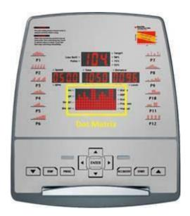
This is a LED display console, and the functions shown include: RPM, SPEED, TIME, CALORIES, DISTANCE, WATTS, LEVEL, dot matrix display of the PROGRAM graph.
