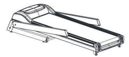
**Step 2:** Insert the upright post into the clamping ring on both sides of the main frame with Allen C.K.S. half head screw M8x50x20 and Allen C.K.S. full thread screw M8x15 (without lock for now).
