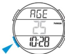
4. Press "D" to increase the number, press "C" to decrease the number, press and hold to adjust at high speed;
