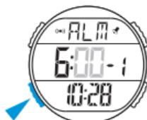
4. Press "D" to increase the minutes, Press "C" to decrease the minutes, press and hold to adjust at high speed;
